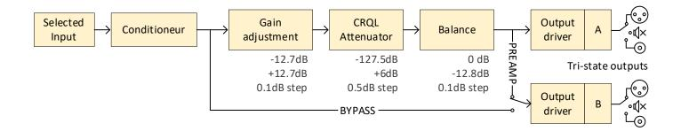
*Output B can operate in two different modes:*
